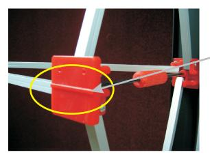
When mounting plastic magnetic channel bars do not cover high point on frame block. If covered frame will not square up properly and panels will not sit evenly on frame.
