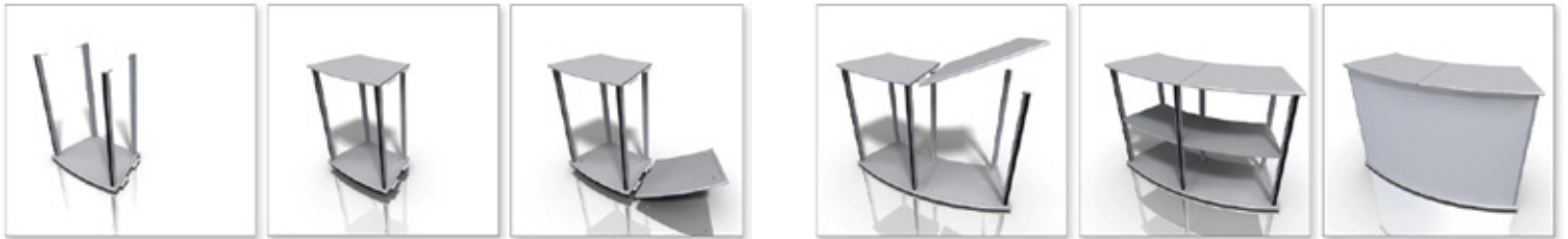
Assemble the first module using the FASTclamp tool-less connector.
