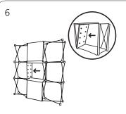
While holding top siding in place, insert left vertical siding. \*Make sure the sides have grooves for shelf.
