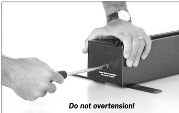
If adjustment is needed, hold the cassette firmly in place then depress and turn the adjusting screw clockwise to increase the tension (the tension mechanism adjusts in halfturn increments). Slowly release pressure on the screw turning slightly counter-clockwise and allow it to again lock in place. If tension has been lost completely, we recommend 20-25 full clockwise turns.
