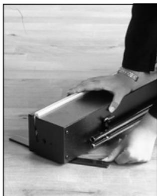
For increased stability pull out the four support legs on the cassette.
