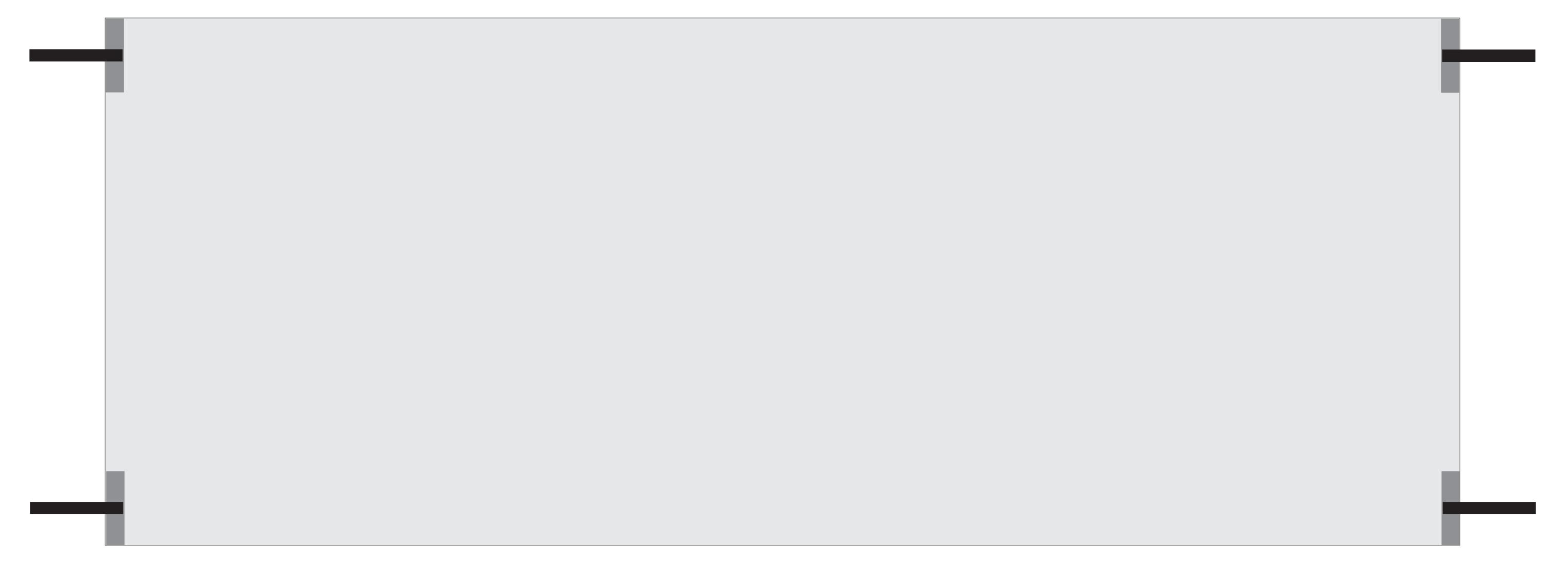
4 velcro strip fasteners mounted in each corner on the reverse side of the graphic panel
