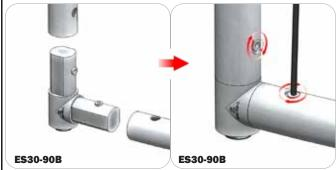
Compress one unlocked end of the connector and slide it through one tube end. Compress the other end of the connector and slide the second tube on. Lock both screws carefully using your hex key tool. Be sure to lock securely, but do not overtighten.
