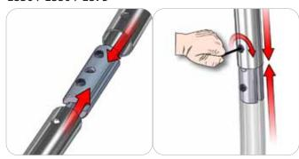
Compress the unlocked connector and slide one tube onto each end. Lock both screws carefully using your hex key tool. Be sure to lock securely, but do not overtighten.
