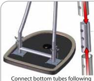
the labels by matching number to number. Slide joiner into tubing so hex screw sits in hole on tubinger.
