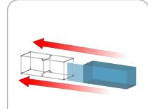
Lay tube frame on its side and pull graphic over frame.
