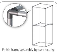
Finish frame assembly by connecting top corners and tubing. \*Frame can be on side for assembly.
