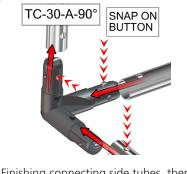
Finishing connecting side tubes, then connect top of frame.
